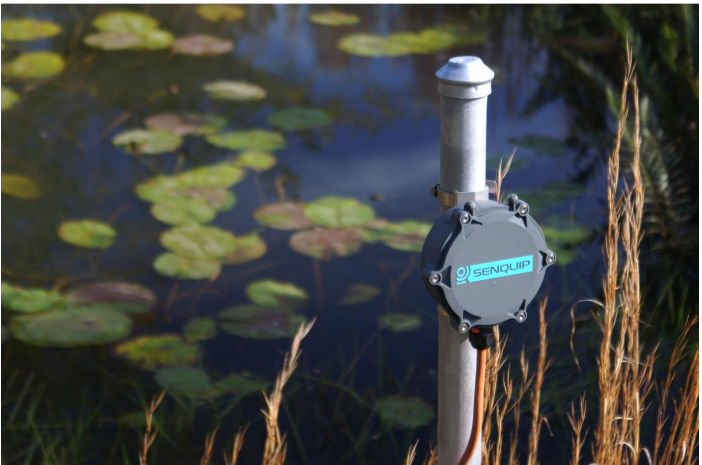
Figure 1 - Battery Powered ORB Monitoring Water Level
