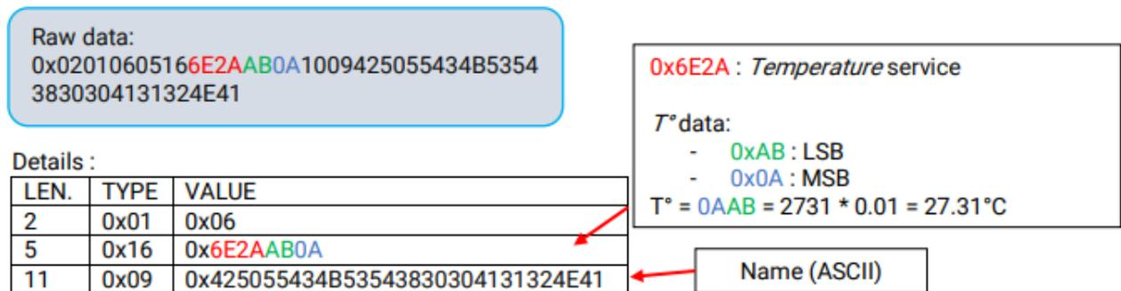
Note: For a negative temperature, data is sent in 2-complement: for example, -27.31°C is 6E2A55F5
