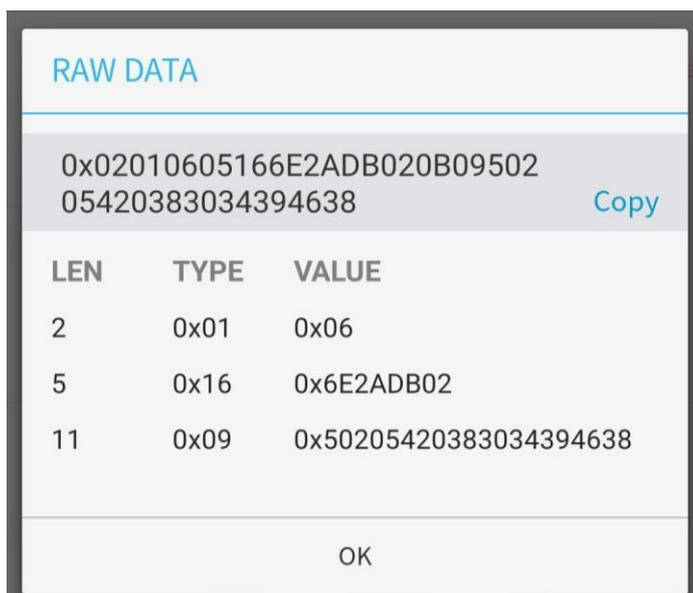
Figure 5 - Raw Data from BLE Temperature Beacon
