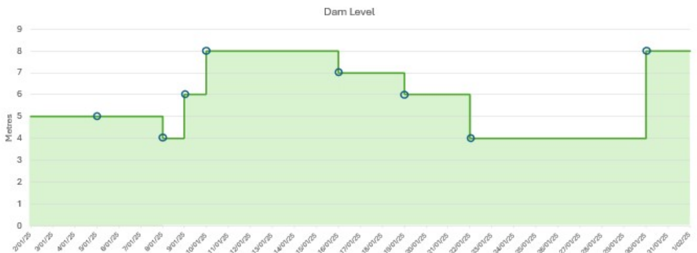
Figure 10.17. Time weighted average works well where there are missing samples
