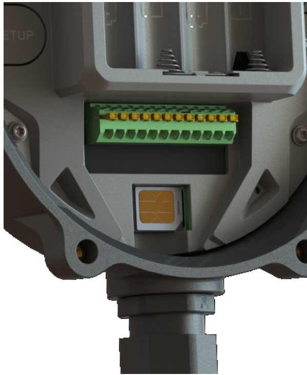
Figure 12.2. Remove the SIM card before opening.
