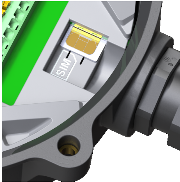
Figure 3.15. Insert SIM to the right
