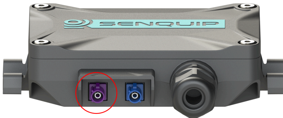
Figure 8.1. FAKRA-D 4G LTE antenna connector
