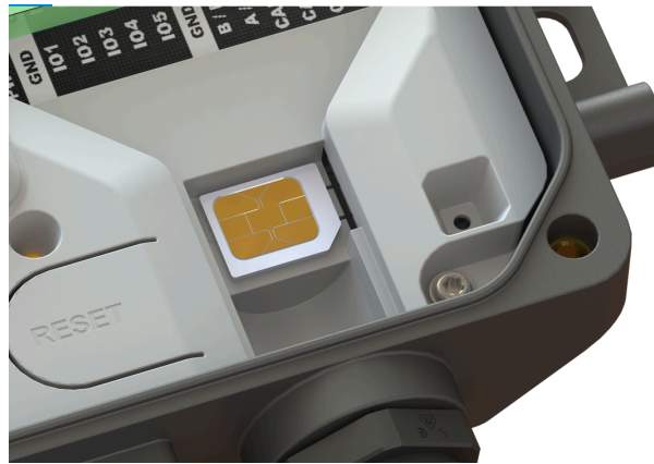
Figure 2.11. Correct insertion of a SIM card
