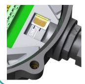
If using GSM and the ORB does not contain an internal SIM, insert a SIM card, note the orientation carefully.
