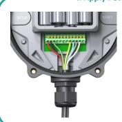
Apply power to pin 1 and ground to pin 2 of the header or insert 4 x AA batteries. The green light will go on and orange light will flash.
