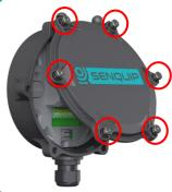
Using the 3mm Allen key provided, loosen the 6 cover screws ensuring that all 6 screws have ejected before opening.
