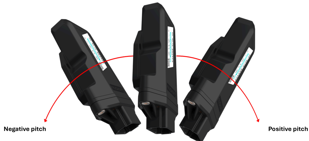
Figure 8.1. Definition of pitch
