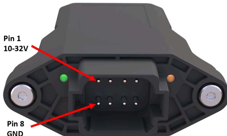
Figure 2.5. UNI-Z1 power connection
